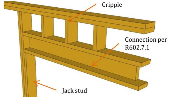
Single member headers shall be framed with a single flat 2" member or wall plate not less than the width of the wall studs on top and bottom of the header.
