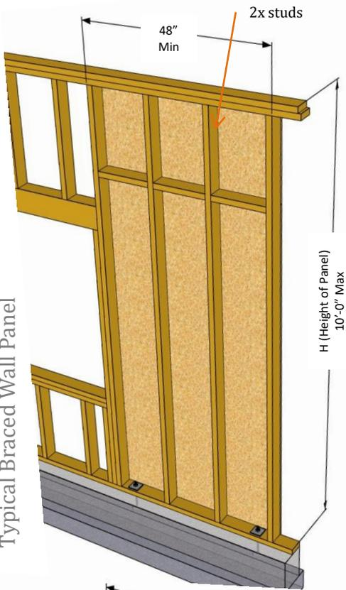
Alternate Braced Wall Panel
