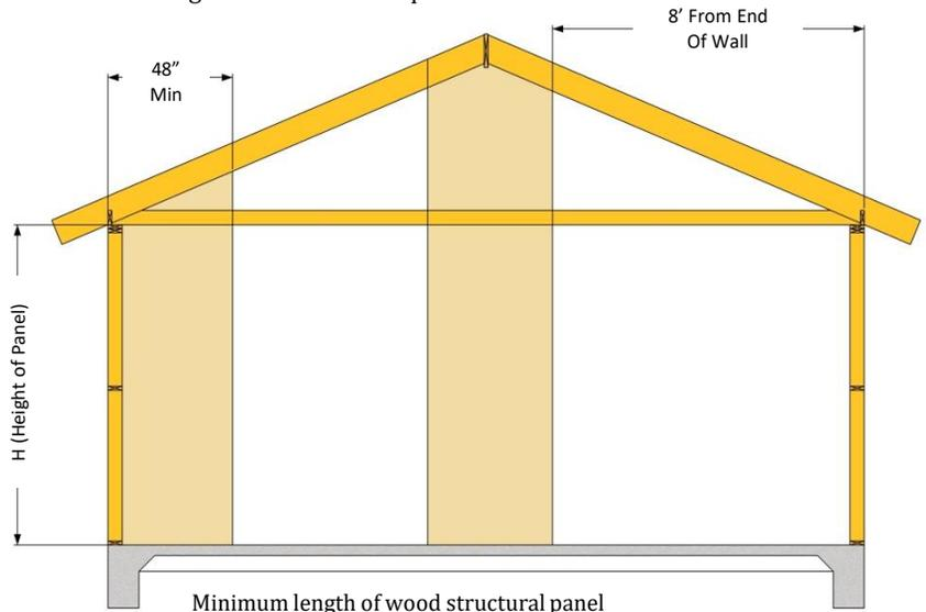
Minimum length of wood structural panel walls: min. 12'-0" of braced wall length for each 25 lineal ft. of braced wall line.
