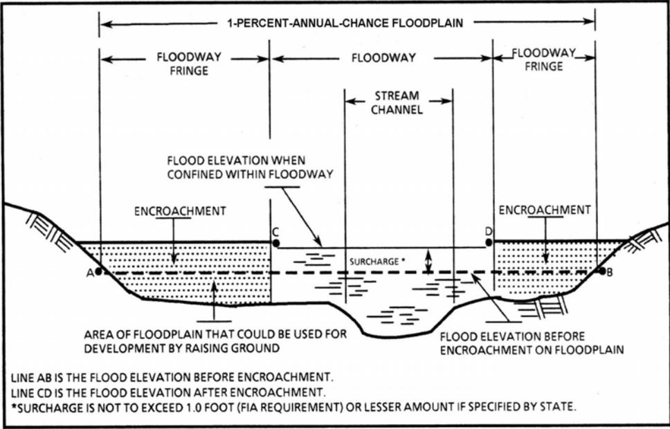
FIGURE 1: FLOODWAY SCHEMATIC
