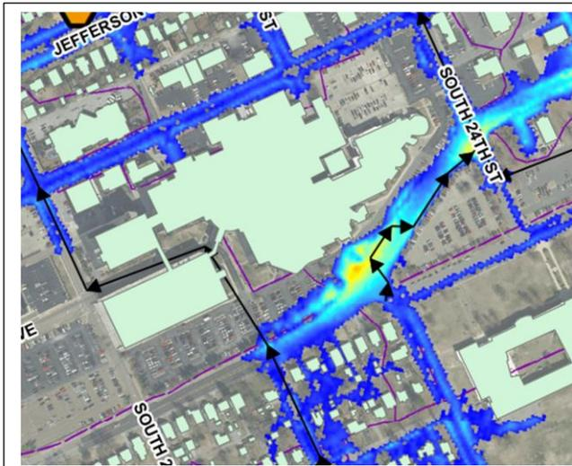
**Figure ES-14 Modeled Flooding at Hospital July 7, 2015**
