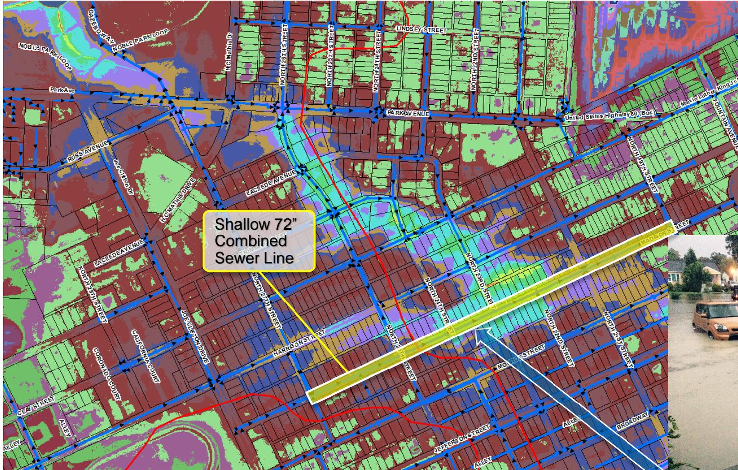
LIDAR Topographic Data Indicates Lack of Overland Flood Route Over Park Ave.
